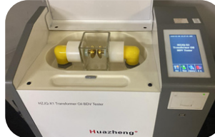
YAĞ DELİNME İZALASYON TEST / OIL BREAKDOWN DI-ELECTRICK TEST
